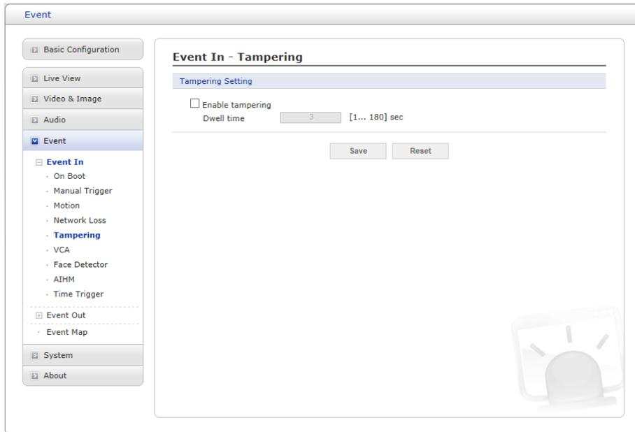
This is used to trigger an event when camera tampering occurs, for example, obstruct the camera with foreign material or move camera direction using external force. Select “Enable tampering” to activate the Tampering event.
