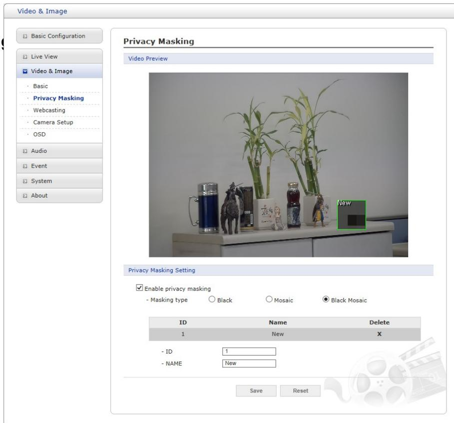
The privacy masking function allows you to mask parts of the video image to be transmitted. You can set up to eight privacy masks and the color of privacy masks is black.
