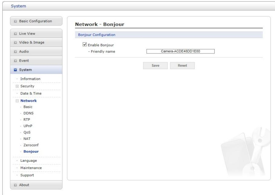
The network camera includes support for Bonjour. When enabled, the network camera is automatically detected by operating systems and clients that support this protocol.
