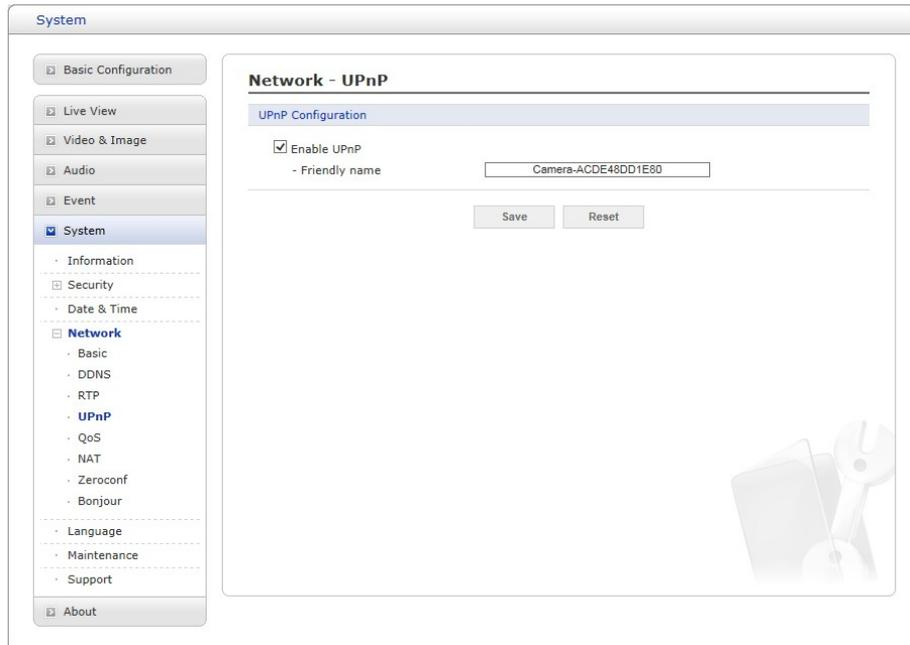
The network camera includes support for UPnP. UPnP is enabled by default, so the network camera is automatically detected by operating systems and clients that support this protocol.
